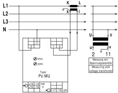
**Type Pnz-MU** (Dreileiterdrehstrom gleich belastet / three-wire three-phase current of same load)
