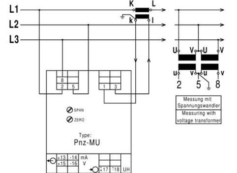
**Type Pd-MU** (Dreileiterdrehstrom beliebig belastet / three-wire three-phase current of any load)
