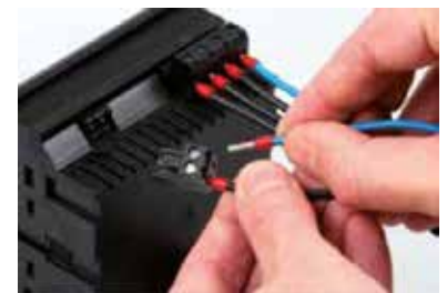
Fig.: Pluggable screw terminals for easy connection
