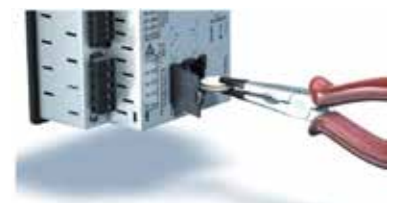
Fig.: Replacing the battery using ling-nose pliers
