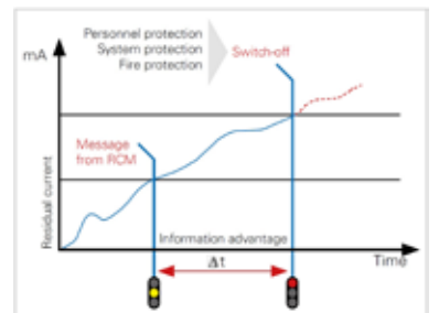
Fig.: Report prior to switching off – an aim of residual current monitoring
