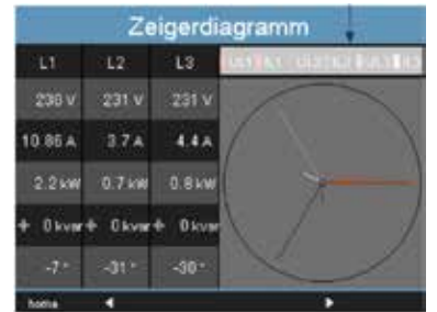
Fig.: Example phase sequence in the vector diagram
