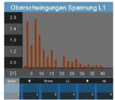
Fig.: Example harmonics voltage L1
