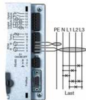
Fig.: Connection example of residual current monitoring and PE via current transformers
