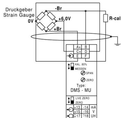
For devices with frequency output further outputs not available. Terminals +13 and -14 are the frequency output.
