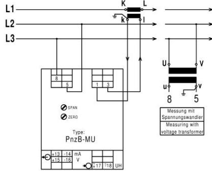
**Type PdB-MU (Dreileiterdrehstrom beliebig belastet / three-wire three-phase current of any load)**
