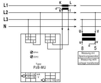
**Type PnzB-MU (Dreileiterdrehstrom gleich belastet / three-wire three-phase current of same load)**
